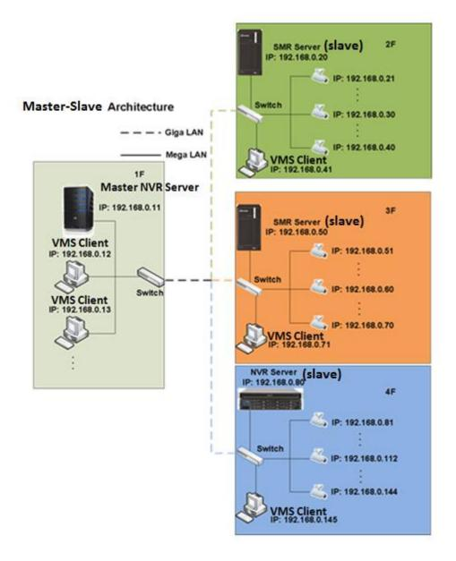
Picture2: The architecture of Master/Slave solution
