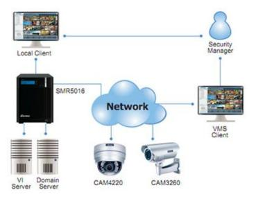
Picture1: The architecture of standalone solution
