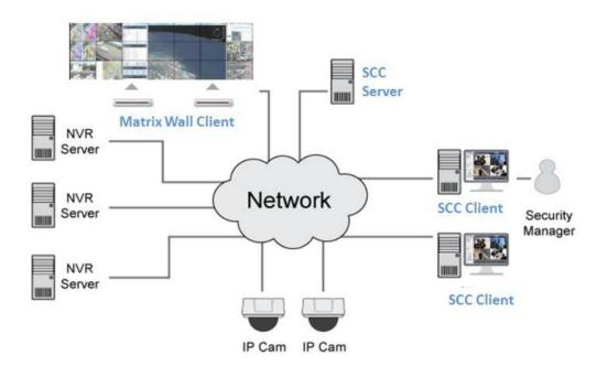
Picture4: The architecture of domain sever solution
