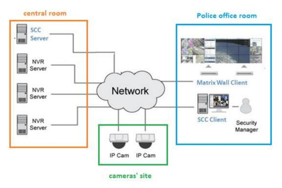
Picture5. The architecture of domain server solution in Mongolian traffic surveillance
